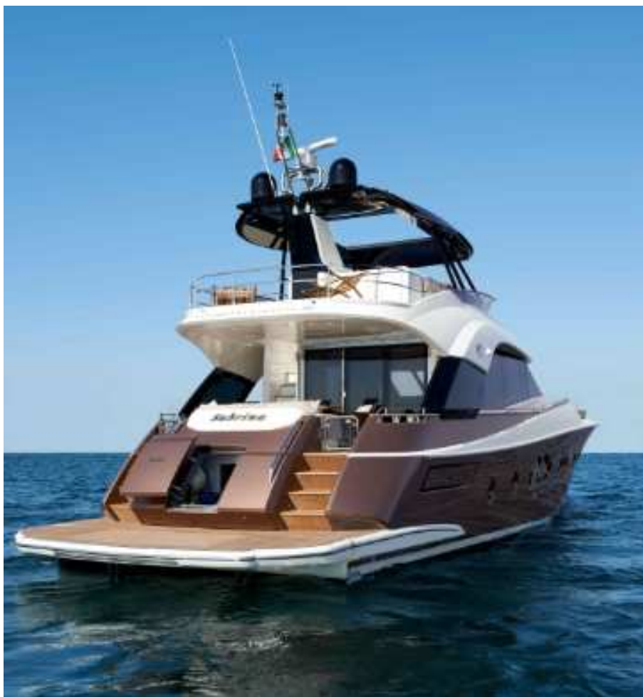
MCY 70: Carbon T-Top with electric opening soft top
